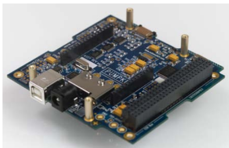
Figure III.6: On-board computer (OBC) subsystem of OUFTI-1
